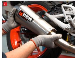
I) OPTIONAL - In the fitting kit we supply a Flute to place between the connecting pipe and the silencer. This is an optional part to reduce the sound level. If you wish to use it now is the time to insert it into the connecting pipe.
