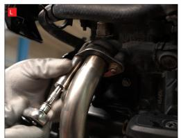
K) Bolt the rear silencer to the original mounting bracket using the suppled hardware and spacer. Use the diagram on the first page to see the order they need to be fitted. Leave slightly loose until the rest of the system has been adjusted and tightened.
