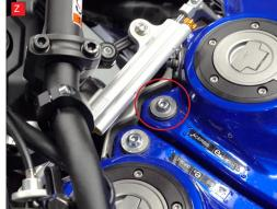
Y) Unclip the cover at the front of the tanks and then remove from the bike.
