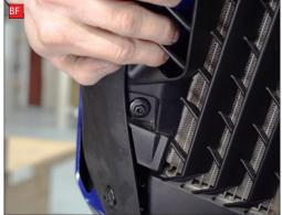
BE) Re-install the front side panel screws, this is the reversal of the removal steps.
