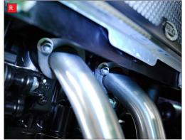
Q) Carefully remove the exhaust system.
