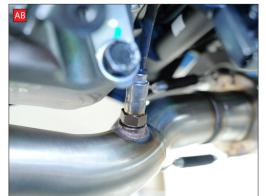
AD) Run both Lambda sensor cables along their original route and secure in place, then reconnect the plugs.
