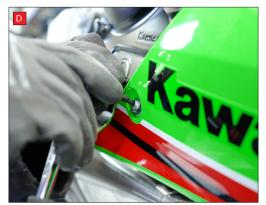
D) Remove the mounting bolt from the lower fairing on the right side of the bike. Support the weight of the fairing as you do so, then carefully remove from the bike once loose.
