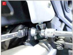
Y) Fully tighten the 4 header nuts.
