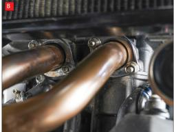
A) Start by removing the lambda sensor from the headers. If you're using a spanner rather than a sensor socket you may find it easier to remove the heat shield first.
