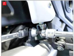
Y) Fully tighten the 4 header nuts.
