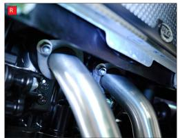
Q) Carefully remove the exhaust system.
