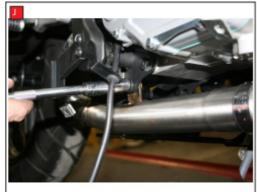
I) Bolt the Scorpion silencer to the O.E mounting bracket and fully tighten. Then fully tighten the bolt that gose onto the Scorpion silencer mounting bracket.
