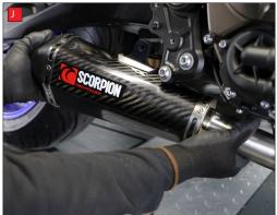
I) Attach the Scorpion mounting bracket to the original mounting point on the frame using the suppled hardware.
