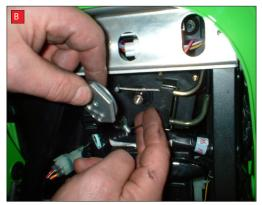
A) To disconnect cables at the seat end, you have to remove the hexagonal wheel, without turning it's shaft.
