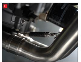
L) Install the springs between the silencer and the collector pipe and between the collector pipe and the header pipes.
