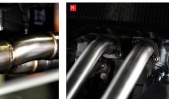
N) Adjust the position of the system to where you're happy that it has clearance around it and there's no stress on any joints, then fully tighten the header nuts, silencer to mounting bracket bolt and mounting bracket to frame bolt.
