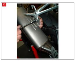
X) Fit the clamp over Scorpion connecting pipe before sliding into position
