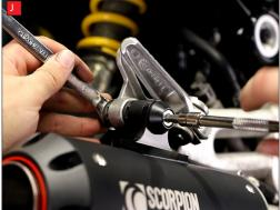
I) Align the system so that it is sitting in the correct position and is clear of any moving parts, then tighten the clamp between the header pipe and the connecting pipe.
