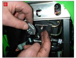
D) Remove hexagonal wheel from shaft, retaining OE bolt.
