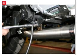
D) Attach Scorpion link pipe to the header pipe, making sure you put the clamp on loose, once sloted in tighten up the lower mounting bracket but only FINGER TIGHT.
