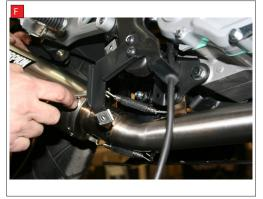
F) Now you can offer the Scorpion silencer to the bike and connecting pipe, slide the silencer into the collar of the scorpion link pipe and attach the rubber coated springs (best tool is a spring puller, we can supply you with this tool)
