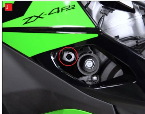
I) Staying on the left side of the bike, remove the lower fixing from the back of the fairing.
