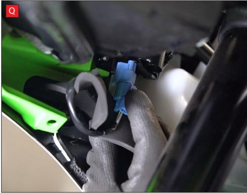
Q) Disconnect the wiring for the indicator.
