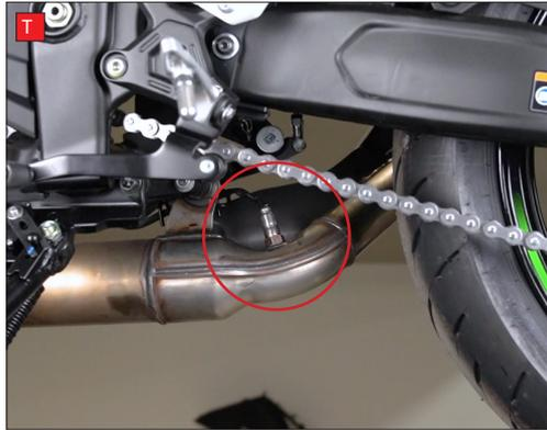
V) Remove the nut and bolt from the silencer mounting.
