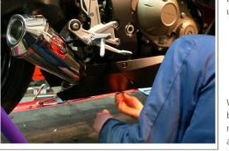
When all the above steps have been completed doble check all nuts and bolts are tight and that all original bike functions are not impaired. When satisfied fitment is correct take your bike for a short run to ensure system is sealed correctly and there are no gas leaks. After a short run, allow your bike to cool and check all nuts and bolts are tight.
