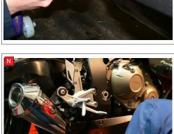
I) Sild the underbelly box onto the original pipework and tighten up the clamp.
