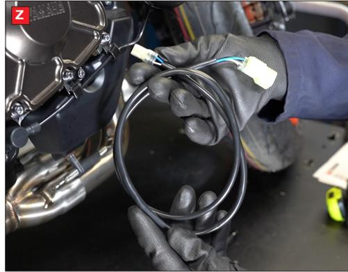
Y) Connect the lambda sensor to the extension cable and neatly secure with the breather pipes.
