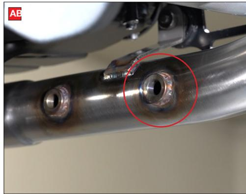
AB) Screw the Lambda sensor into the Lambda Catalyst, then screw the Lambda Catalyst into the rear boss on the Scorpion connecting pipe. Use the supplied copper washer and fully tighten the assembly.
