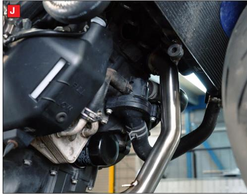
I) Using the diagram on the 1st page, install the new mounting bracket with the supplied hardware. Leave the bolts loose to allow adjustment, you will fully tighten them in a later step.
