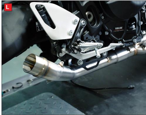
L) Fit the connecting pipe to the collector. Use the original bolt to secure the pipe to the bike.
