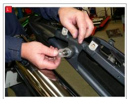
M) Ensure that the Scorpion system is sitting level and square and that none of the original functions of the bike are impaired.
