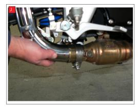
J) Introduce the Scorpion connecting pipe CP 436 to the header pipe with the clamp on the CP 436.
