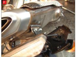
S) Re-fit lower seat fairing, using the supplied 2 x M6x25mm screws and washers in the 2 furthest back holes.
