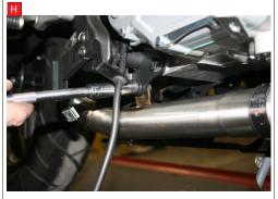
H) Fully tighten the lower mounting bracket and the clamp that fixes the header pipe and the link pipe together.
