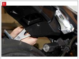
Q) Fit the Scorpion composite fairing, using the line drawing on page 1 to make sure all the fixings are in the correct place, on the top mounting point on the fairing use the O.E bolt.
