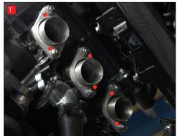
T) If your header gaskets are in good condition you can reuse them. If they're not you should replace them now with Triumph part number T2200854. Loosely bolt the collars to the engine ports using the flanges so that the collar still has movement during installation. Ensure the holes on the outside flanges are to the bottom and the holes on the middle flange is to the top.
