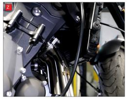
Y) Install the remaining springs between the spring hoops.
