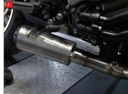
I) Attach the Scorpion mounting bracket to the original mounting point on the frame using the suppled hardware.
