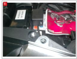
A) Remove seat, remove right hand side panel as shown in pictures A & B.
