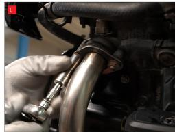
K) Bolt the rear silencer to the original mounting bracket using the suppled hardware and spacer. Use the diagram on the first page to see the order they need to be fitted. Leave slightly loose until the rest of the system has been adjusted and tightened.
