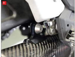
Q) Slide the silencer onto the connecting pipe.
