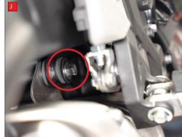
I) Remove the bolt that attaches the gear selector to the bike. This is to give you access to the exhaust mounting bolt behind it.
