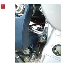
A) Remove the cover off the Exup Valve
