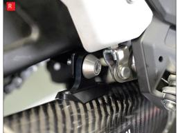
Q) Slide the silencer onto the connecting pipe.
