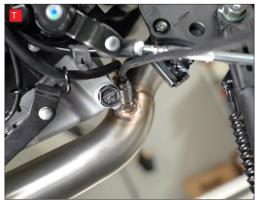
T) If your bike has a 2nd lambda sensor, screw it into the rear sensor boss on the connecting pipe and fully tighten (25Nm/18ftlb). Route the cable along its original path and reconnect the plug. If your bike only has 1 lambda sensor, use the supplied blanking plug and copper sealing washer in the 2nd sensor boss.
