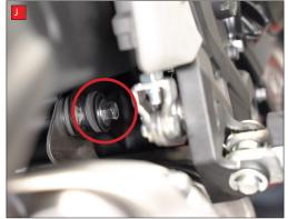
I) Remove the bolt that attaches the gear selector to the bike. This is to give you access to the exhaust mounting bolt behind it.
