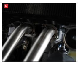
N) Adjust the position of the system to where you're happy that it has clearance around it and there's no stress on any joints, then fully tighten the header nuts, silencer to mounting bracket bolt and mounting bracket to frame bolt.
