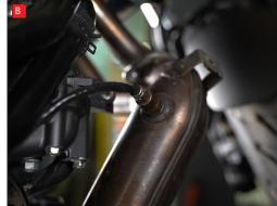
A) Start by removing the 2 screws from the catalytic convertor heat shield to allow you to remove it from the bike.
