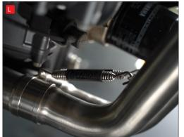
L) Install the springs between the silencer and the collector pipe and between the collector pipe and the header pipes.
