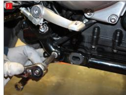
I) On the left side of the bike unbolt the two bolts joining the frame at the rear.
