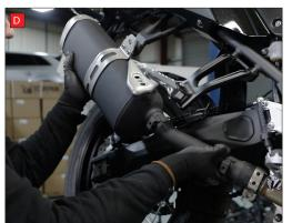
D) Carefully remove the silencer from the bike. If the gasket stays on the original centre section remove it as it's not required with the Scorpion headers.
