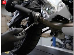
A) If fitting at the same time as the Scorpion Slip-on start by removing the heat shield from the original exhaust.
