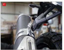
U) Slide the silencer onto the connecting pipe. You do not need the gasket.
