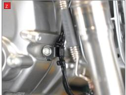
Y) Screw the front Lambda sensor into the boss on the header pipe and fully tighten.
