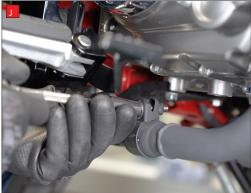
I) Remove the lower mounting bolt for the silencer.
