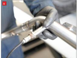
Q) Remove the header pipe from the bike.
