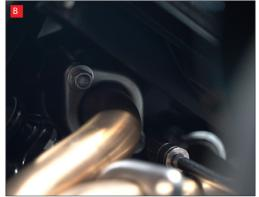
A) Remove the lambda sensor from the exhaust pipe. It is located on the collector at the front of the bike.
