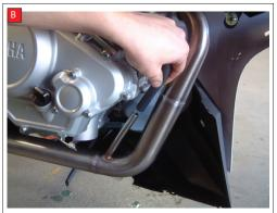
A) Remove all 3 R/H side body panels and remove the O.E exhaust taking care not to lose any of the original fittings. Attach Scorpion front pipe only
