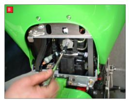
A) Disconnect cables on exhaust valve and leave loose.
