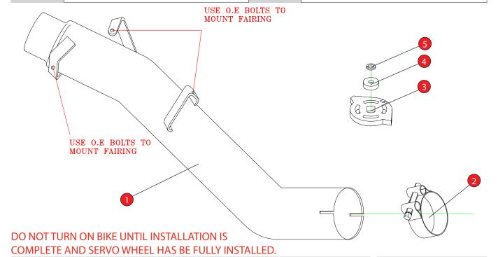
NOTE: ENSURE SCORPION SYSTEM IS CLEAR OF MOVING PARTS AND ALL ORIGINAL FUNCTIONS WORK CORRECTLY.
