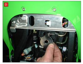
C) The replacement wheel comes with an aluminium coler that is secured in place with O.E bolt and split washer. TIGHTEN TO 5ft/lb USING A TORQUE WRENCH.
